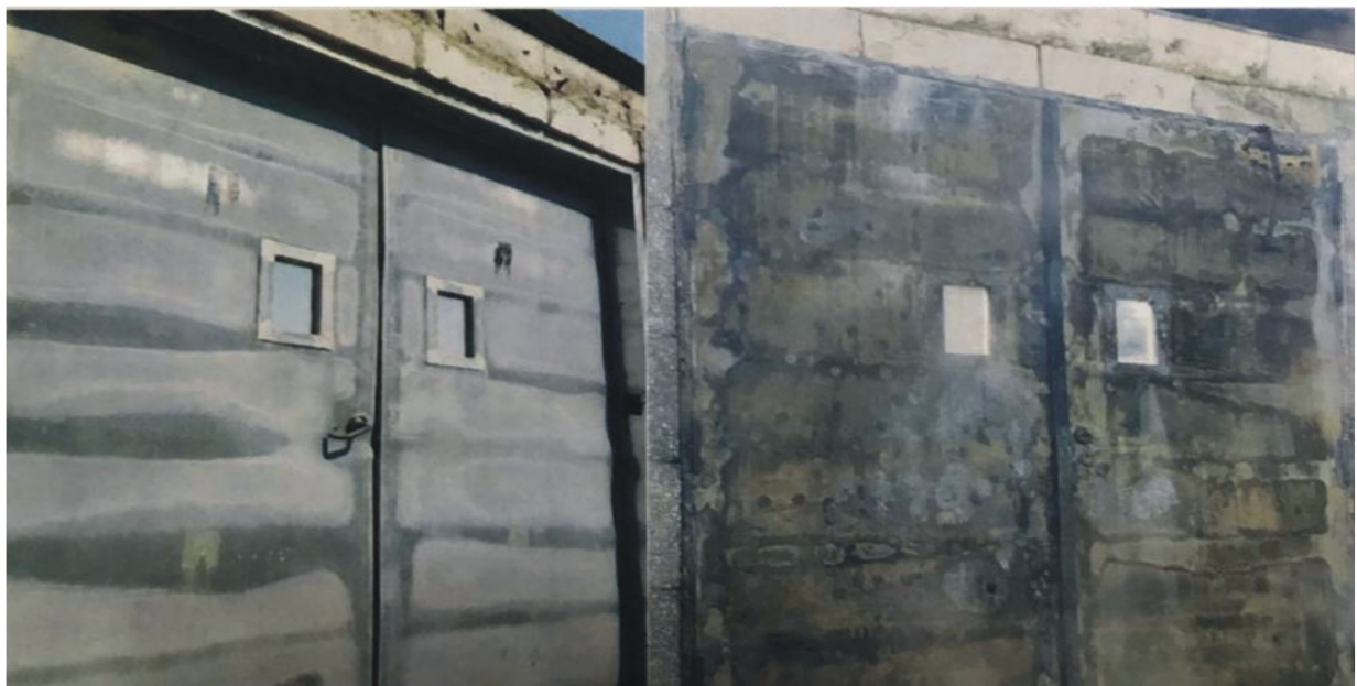
Specimen exposed & unexposed sides immediately after being subjected to hose stream test
