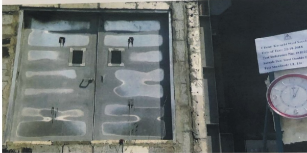
Specimen after 30mins of testing
