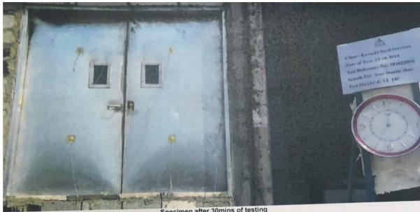
Specimen after 30mins of testing
