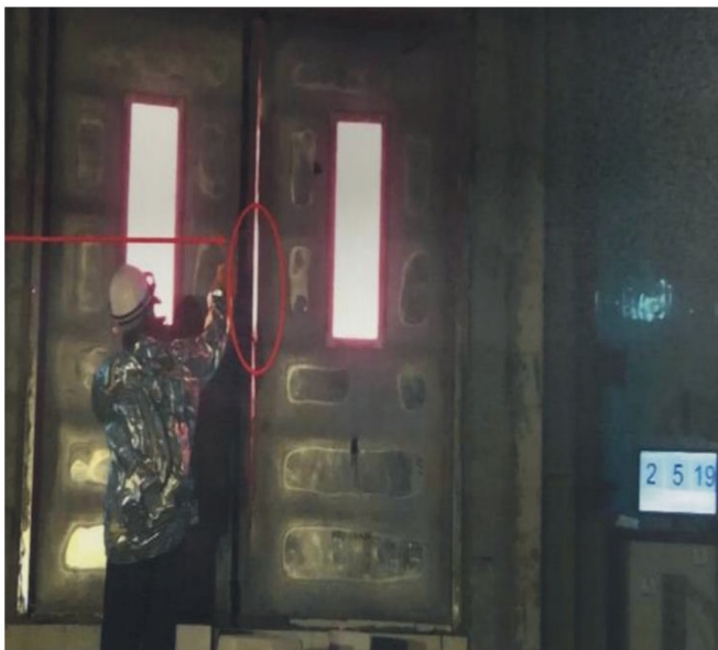
Test failure at 125 Minutes
