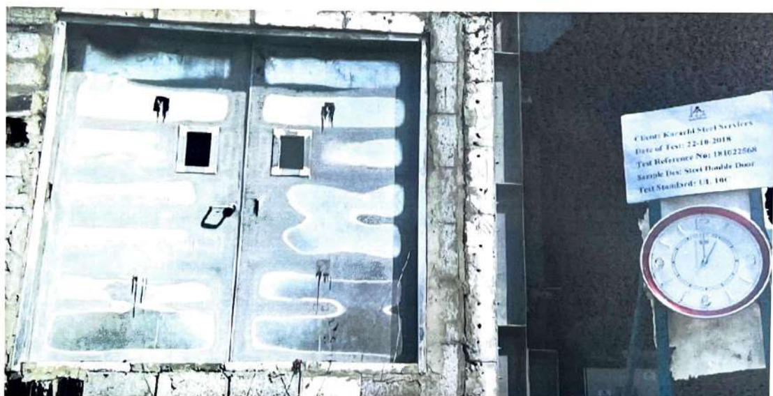
Specimen after 60mins of testing
