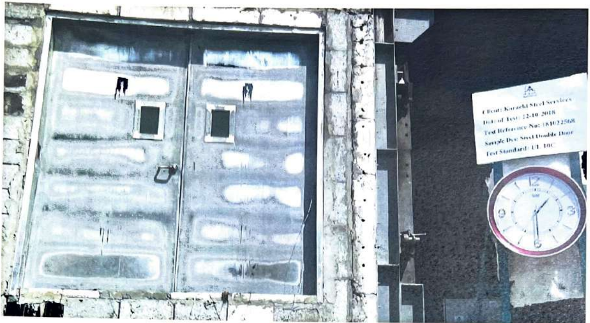
Specimen after 90mins of testing
