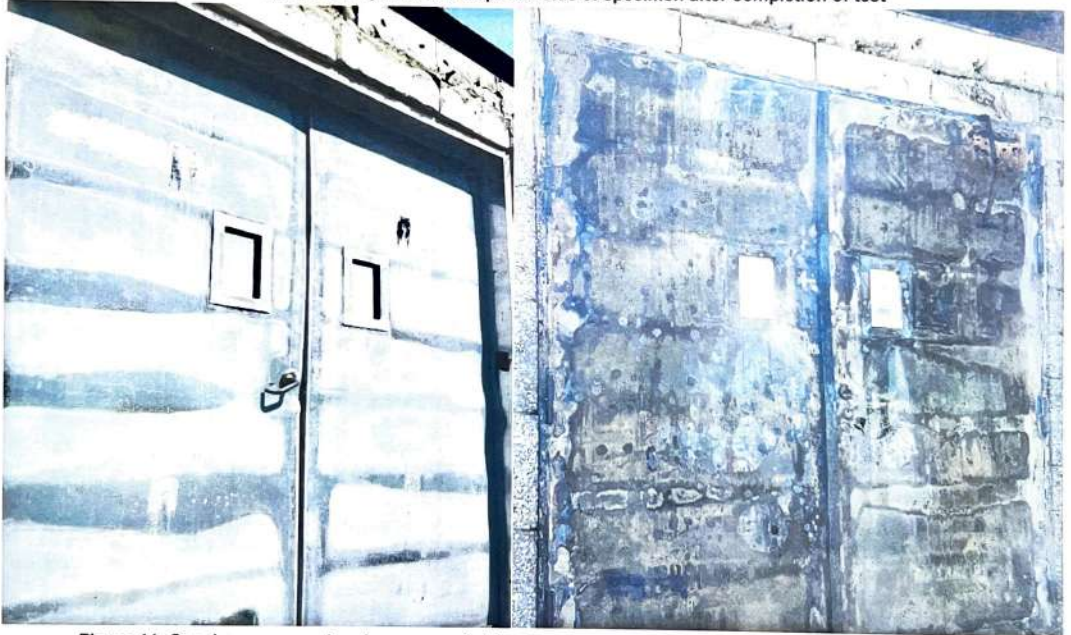
Figure 11: Specimen exposed and unexposed sides immediately after being subjected to hose stream test
