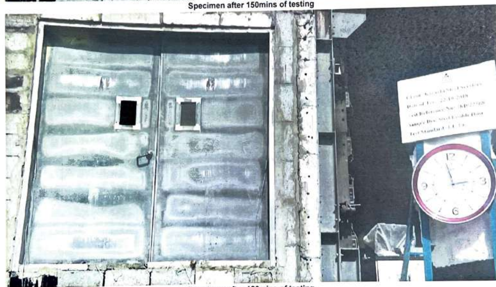
Figure 9.3: Unexposed side of specimen during exposure to fire
