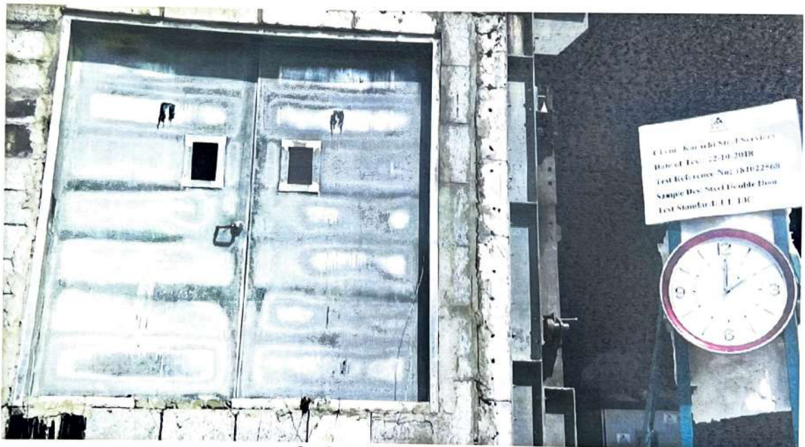
Specimen after 120mins of testing
