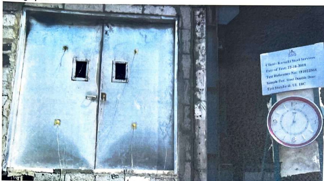
Specimen after 30mins of testing
